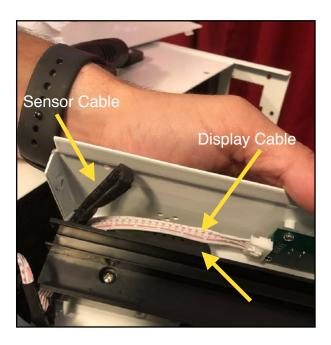
9. Once you've attached the control panel, Make sure to tuck the wires in, so the filters will slide in properly.
