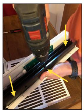
7. Unplug the display cable, then remove the 4 screws holding the display on the control panel. Lift out the display board.
