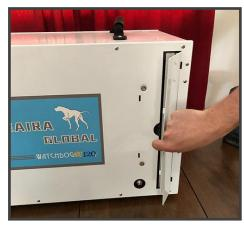
2. Slide out the MERV-10 filter and set it aside (MERV-10 filters come standard on the dehumidifier but you may have a carbon filter or HEPA filter).
