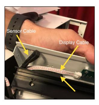
11. Once you've attached the control panel, Make sure to tuck the wires in, so the filters will slide in properly.
