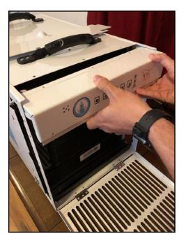
6. Remove the 3 screws on the filter rails to access the sensor. Remove the filter rails from the control panel and set the control panel aside.
