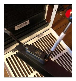
8. Use a flathead screwdriver to carefully open the sensor cover. Set the cover aside.
