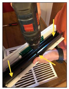
7. Remove the screw on the sensor cover.
