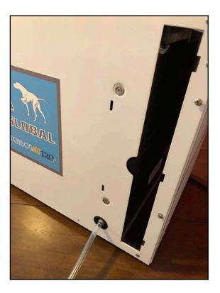
5. Slowly pour the cleaning solution into the drain tray, moving from side to side to evenly distribute it. *NOTE: If you get any cleaning solution on the coils, flush with water.*
