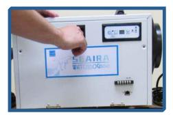
5. Next, use the screwdriver or drill to replace the two screws holding the cabinet door in place.
