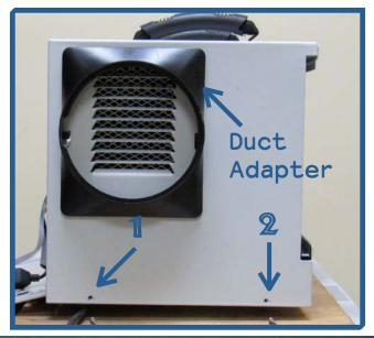
3. Next, replace the 3 screws on the drain hose side of the machine.
