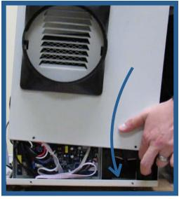
2. Next, you will need to secure both sides of the cabinet. Start by replacing the 2 screws on the duct adapter side of the machine.
