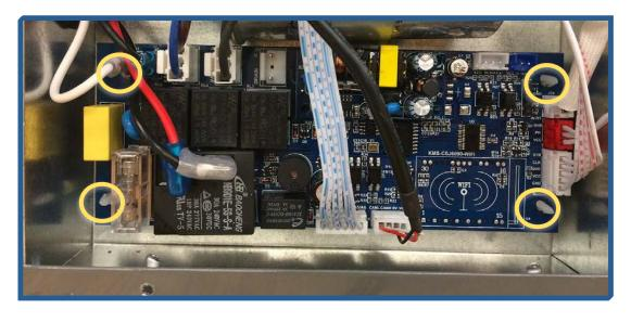
4. Now you're ready to set the old control board aside and insert the new one. Carefully set the replacement control board in place, ensuring the tabs secure into place.
