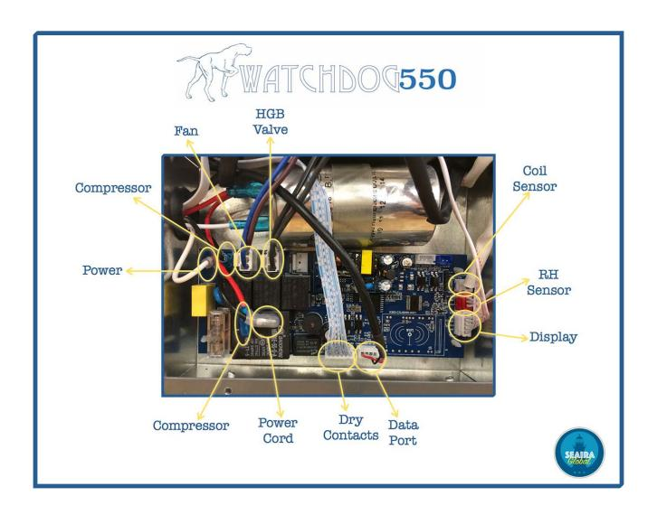
3. Once the wires are unplugged, you can lift the the control board out of the machine. To do this, you will need to the needle nose pliers. Use the pliers to push in the 4 "arrowhead" tabs (one in each corner). Simply squeeze each tab with the pliers so the control board can be lifted over the tab.
