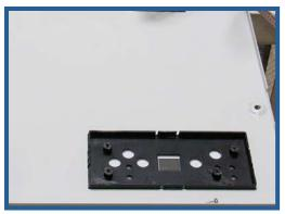
5. Set the old control board aside and grab the replacement control board. Position the control board on the cabinet, then screw into place (remember there are 4 screws, one in each corner).
