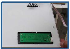
4. Now you can finish removing the display board by unscrewing the 4 screws, then lifting off of the cabinet.
