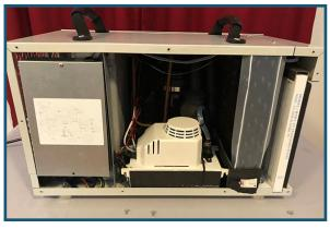
3. Use the quick connect to remove the drain tube from the pump.
