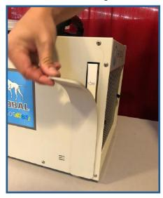
2. Pull on one of the black tabs to remove the prefilter.
