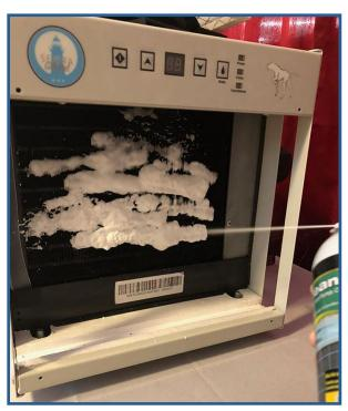
5. Reassemble the unit. There's no need to rinse the coils as the dehumidification process will do that for you.
