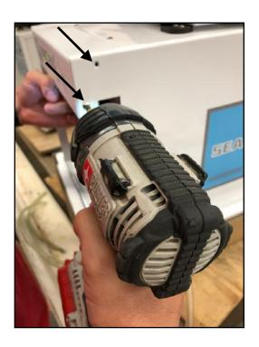
3. Next, remove the two screws on the top of the display, using your hand to keep the display from falling out.
