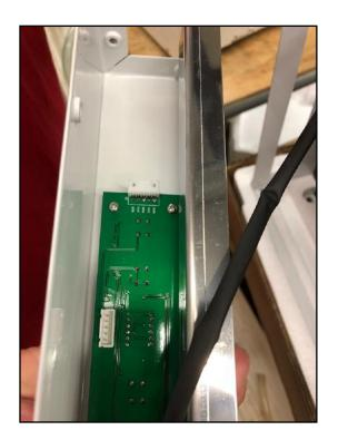
6. Remove the four screws holding the display board in place (2 on each side).
