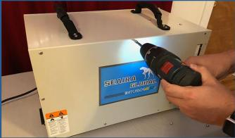
5. Lift off the side panel. Repeat on the other side, if necessary.
