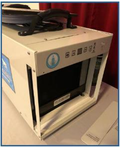
4. Remove the screws holding the side panel in place.
