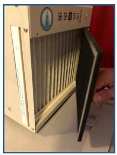
4. Slide out the MERV-10 filter (the MERV-10 filter comes standard on the unit but you may also have a carbon or HEPA filter).
