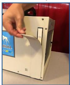
3. Pull on one of the black tabs to remove the prefilter.
