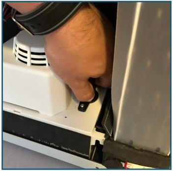
4. Next, remove the two screws holding the pump head in place, using a Philips head screwdriver.
