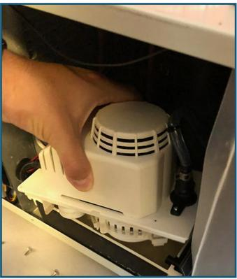
6. Wipe the base of the pump clean using paper towels.
