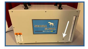
5. Next, remove the two screws on the control board cover.
