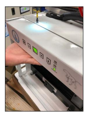
4. Carefully lift the display away from the cabinet and turn it over so you can see the display board. Keep in mind the display will be still be connected by wires to the dehumidifier.
