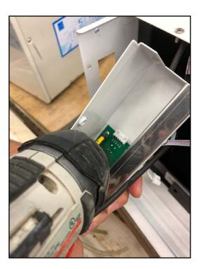
7. Screw in the new display board and reverse the process.
