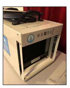
2. Remove the (4) screws on the side of the display. There will be 2 screws on each side.
